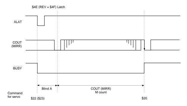
Fig. 2-23 (b). M-Track Move Timing Chart
