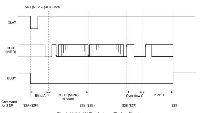
Fig. 2-21 (b). 2N-Track Jump Timing Chart
