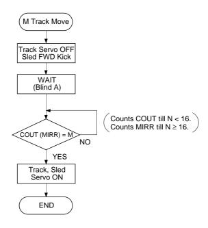
Fig. 2-23 (a). M-Track Move Flow Chart
